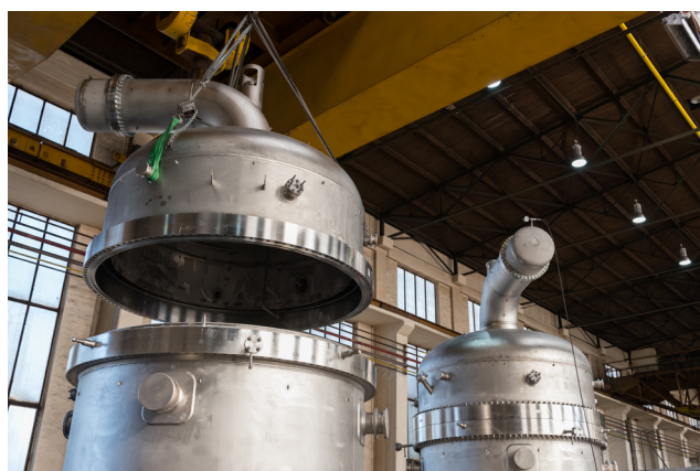
Figure 2. NH 3 waste heat boiler during manufacturing.
